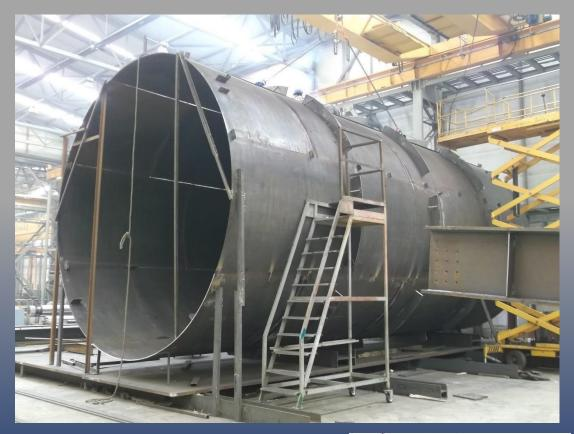
Customer: Spx Belgium Remarks : Fabrication of steam ducts of the power plant in South Africa, 400 tons. Date of completion: 2013
