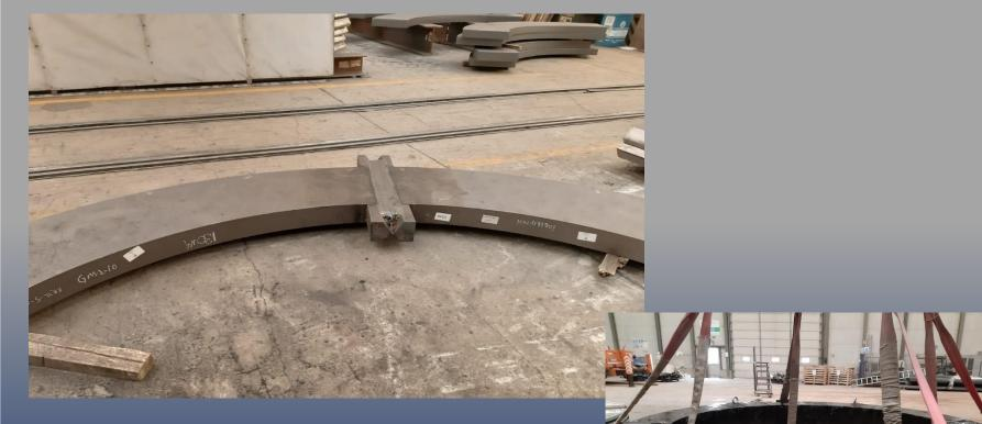
Customer: SIEMENS GAMESA TURKEY Remarks : Fabrication of foundation flanges for wind turbine towers.
