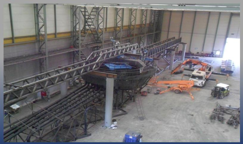
Customer: DEGREMONT SA France Remark: Fabrication of sewage treatment plant. Date of Completion : 2013
